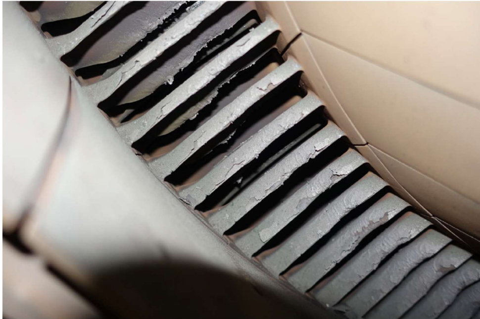
LPT S3 Vane, Thermal Damage and Vane Coating Flaking
