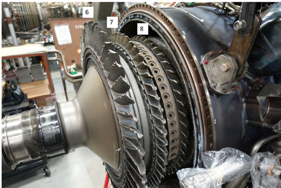
HPC S6, S7 and S8 damage
