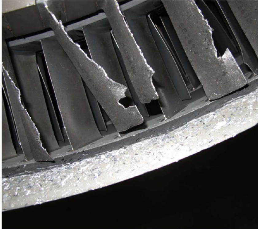
LPC S4 Rotor Blades – Trailing Edge Damage, Blade Tip Separation
