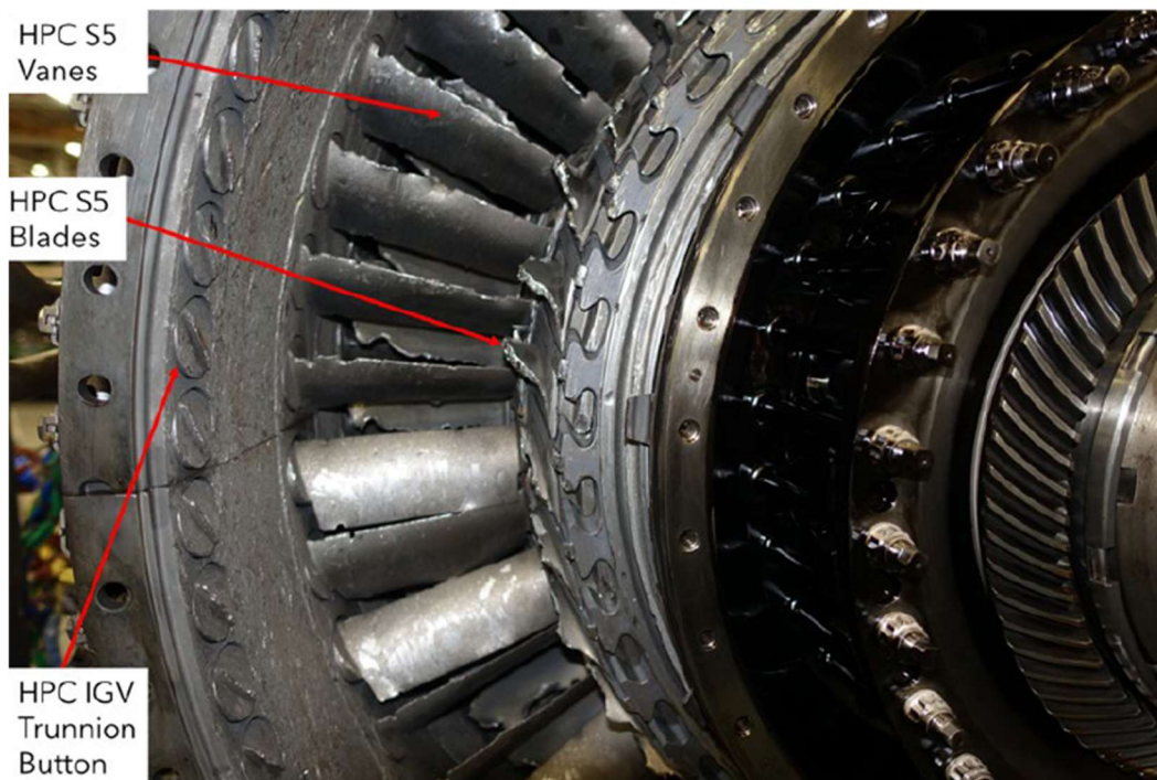
HPC IGV Trunnion Buttons, HPC S5 Blade Fractures, HPC S5 Vanes
